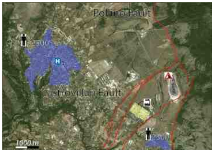
Fig. 2 – The Castrovillari and Pollino faults in Northern Calabria directly run very close to critical facilities and densely populated villages.
