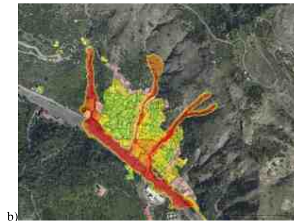
Fig 4 - Images of vulnerability map for Giampilieri village: a) developed using FLO-2D; b) comparison between FLO-2D results and these coming from the speeditive approach.
