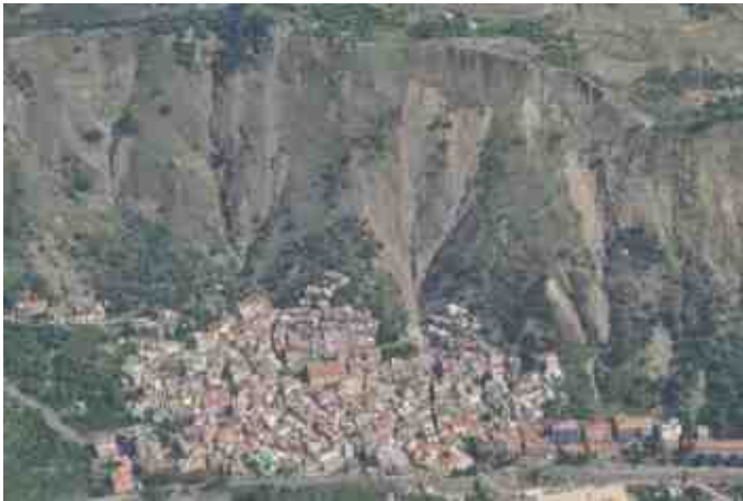
Fig. 2 – Aerial view of the shallow debris slides/debris flows occurred upslope the village of Giampileri.
