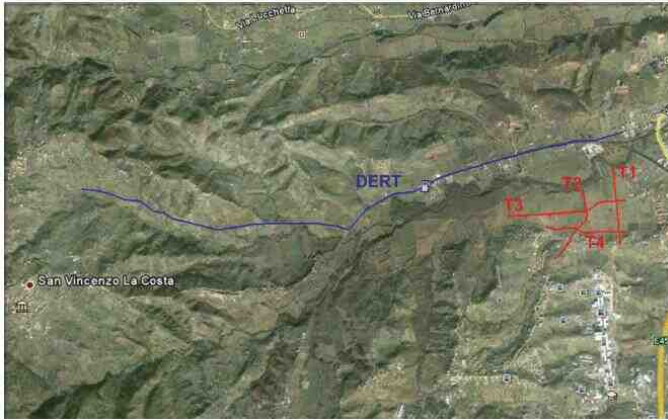
Fig. 5 – The Arcavacata study area: profiles of the geo-electric high-resolution tomographies (T1, T2 T3 e T4, in red) and of the deep tomography (DERT, in blue) performed by CNR-IMAA.
