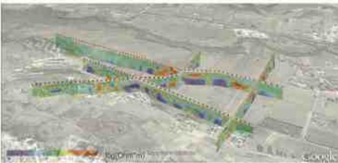
Fig. 6 – Preliminary results of superficial geo-electrical tomography (view from the South).
