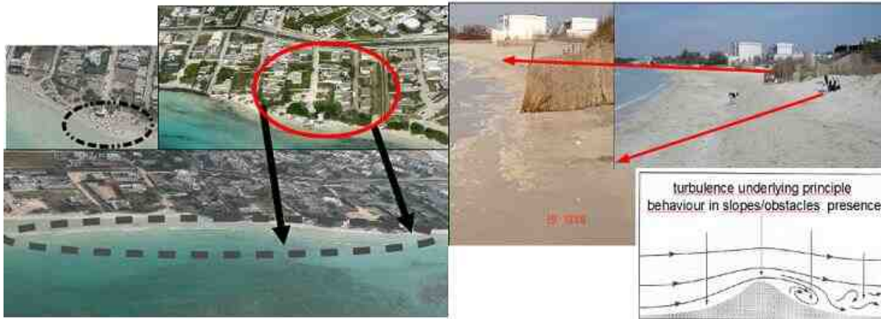
Fig. 2 –Area before erosion on the left high corner adjacent picture coastal in erosion phase red circled. Intervention area and barrier line grey dashed line. A particular of sand deposition after experimental intervention and turbulence effect after slopes on the right.
