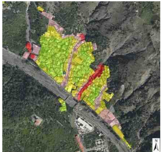
Fig. 3 - Color-coded hydrogeological risk map of Giampilieri Town, developed using a speditive approach.
