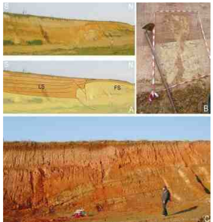
Fig. 2 - On the top of Monte Netto, 10 km S of Brescia, new quarry works in 2007 exposed a Late Pleistocene to Holocene fluvial (FS) and loess (LS) sequence affected by growth folding and surface faulting and seismic induced liquefaction features (B).
