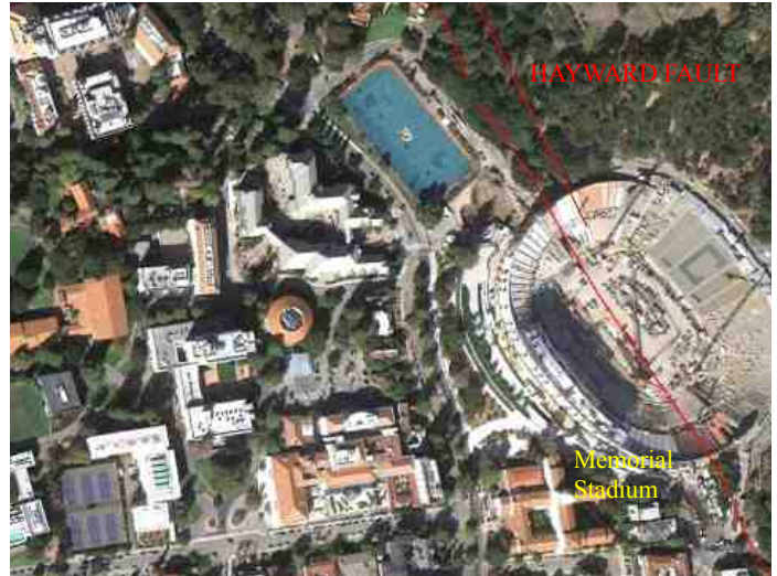
Fig. 1 – On the Berkeley campus, the Hayward fault is well-known for running from "goal post to goal post" in Cal Memorial Stadium.
