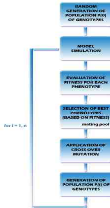
Fig. 2 – Steps of the Genetic Algorithm for model calibration.
