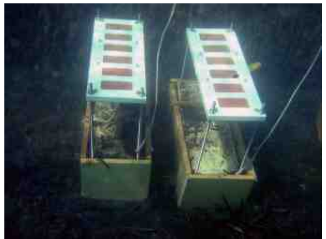
Fig. 1– Ertacetal® cover shields with ceramic briquettes kept in open underwater environment characterized by oxidizing conditions.
