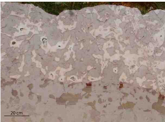
Fig. 2 – Megalodont and Triasina wackestone pervaded by spongy-like dissolution. The part below is filled by reddish silt while the part above by cements. Quarry A at Monte Sparagio, near Custonaci.
