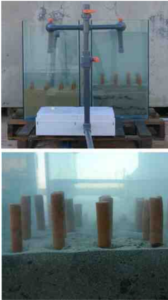
Fig. 2 – Ceramic cylinders placed in custom-made glass containers with two different types of bottom sediment.
